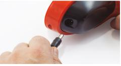
1. Connect the IONIZER PRO gun to the charger.
